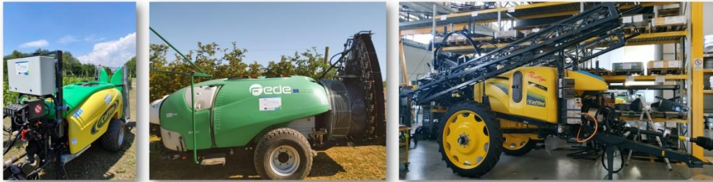
Figure 5. The smart sprayers (for vineyards, apple orchards and open field carrots respectively)
